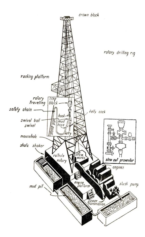
The kelly or kelly joint or grief stem is the top section of the drilling string. Each time a bit becomes dull and needs replacement, the entire string of pipe has to be pulled from the hole and re-run. To save time, the pipe is generally pulled in doubles (two joints at a time) or trebles (three joints at a time) and stacked upright in the derrick in rows called stands. Going in or out of the hole with the drill pipe is called a trip. A complete "in and out" job is referred to as a round trip.
