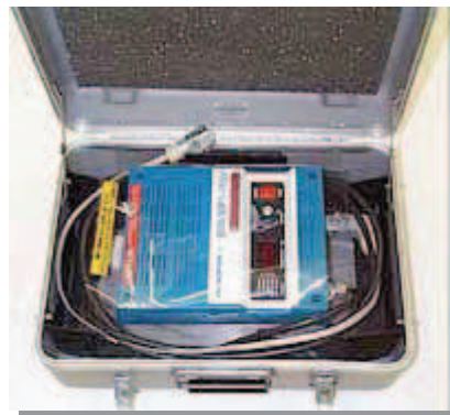
Figure 32: These types of monitoring equipment can be very sophisticated and costly. Automated samplers and recorders however, can be programmed to collect valuable information on a continuous basis or during certain conditions. This makes them important tools for stormwater or flow studies.
